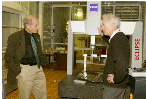
Figure 7: Prof. J.Cronin has inspected the special tool ECLIPCE for precise 3D-measurements of the mold and Fresnel mirror segments.
