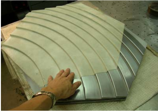
Figure 5: The steel mold and skin plate that is used for fabrication of the reflective superlayer.
