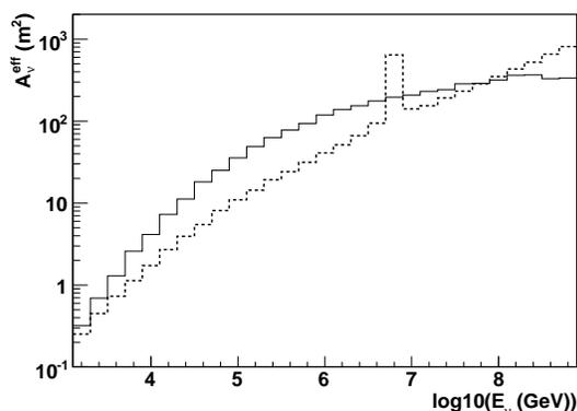
Figure 1: IceCube’s effective neutrino area as a function of the neutrino energy at trigger level for  $\nu_{\mu}$  (solid) and  $\nu_e$  (dashed). The  $\nu_{\mu}$  effective area is the average for neutrinos from the northern sky ( $2\pi$  sr) whereas that for  $\nu_e$  is averaged over the whole sky ( $4\pi$  sr). The peak at 6.3 PeV is the Glashow resonance.
