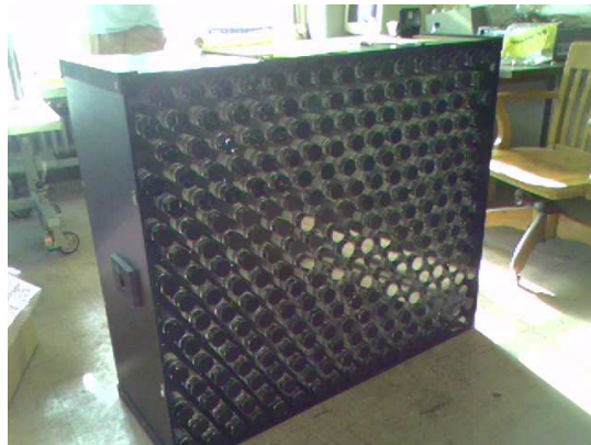
Figure 4: A picture of the assembled PMT cluster box awaiting the addition of the Winston cone frame.
