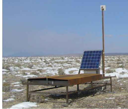
Figure 2: A photograph of a SD deployed in the field. SDs are carried from the accumulation place in several places to each coordinates position by the helicopter.
