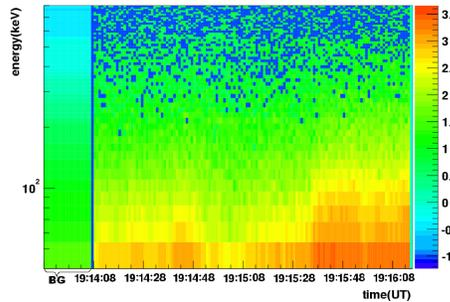
Figure 4: The observed spectrogram of SF010406. Energy in log scale versus time(UT), the color indicates the counting rate per channel in log scale. The left side is the background spectrum for comparison.
