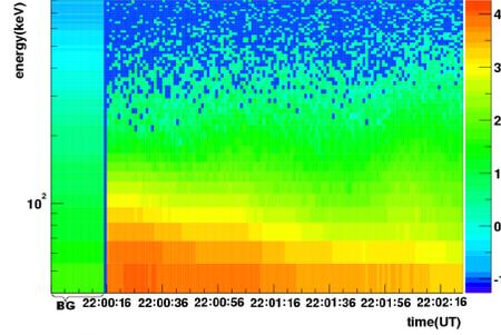
Figure 3: The observed spectrogram of SF010402, Energy in log scale versus time(UT), the color indicates the counting rate per channel in log scale. The left side is the background spectrum for comparison.
