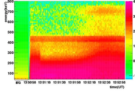
Figure 6: observed spectrogram of SF010415, Energy in linear scale versus time(UT). the color indicates the counting rate per channel in log scale.
