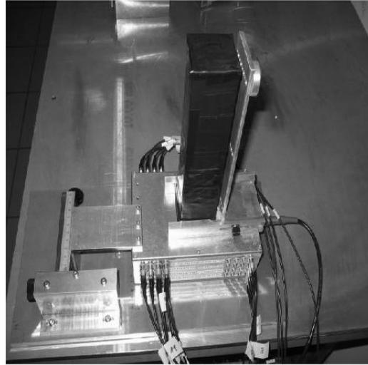
Figure 3: Single POLAR laboratory module with the 8x8 MAPM H8500 coupled to 6x6x200 mm<sup>3</sup> plastic scintillators.
