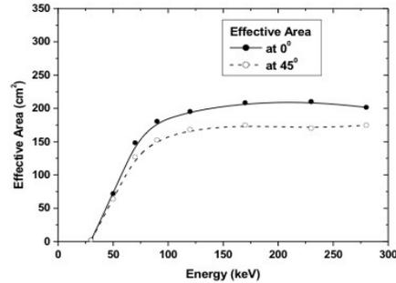
Figure 1: Detector effective area as a function of energy for photons coming at two different polar angles  $\theta=0^\circ$  and  $\theta=45^\circ$  (azimuth angle  $\phi=0^\circ$ ).
