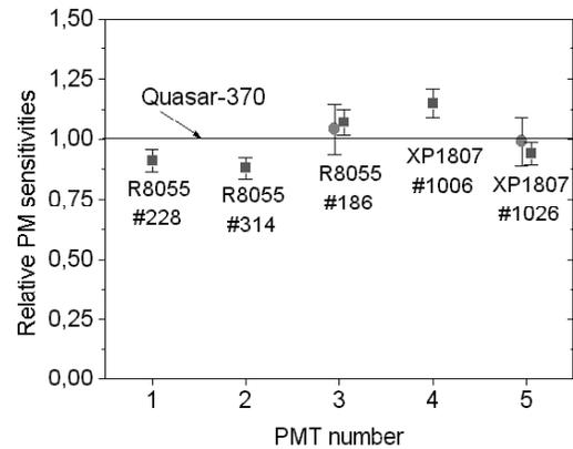
Figure 4: Ratio of effective sensitivity of large area PMs R8055/13" and XP1807/12" to QUASAR-370/14.6". Laboratory (squares), in-situ (dots).
