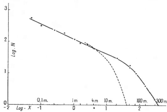
Fig. 6. Decoherence curve measured by Auger at high altitude. The dashed curve is the measurement in the Paris laboratory.
