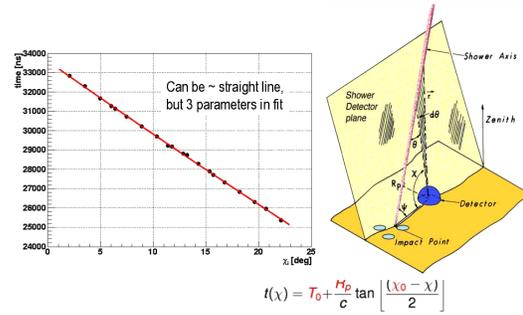
Fig. 30. On the left: plot of signal arrival time vs angle of each pixel. On the right: diagram of the geometrical quantities concerned with the fluorescence reconstruction. On the bottom: the equation relating the quantities to be determined in the geometrical reconstruction.
