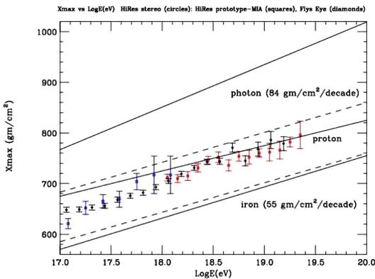
Fig. 25. The elongation rate measured by Fly’s Eye and HiRes. The solid and dashed curves represent the expectations for two different interaction models. Photon induced showers are expected to penetrate much deeper.
