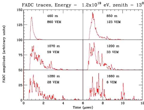
Fig. 13. FADC traces from a single event showing the time spread of shower particles as a function of distance.
