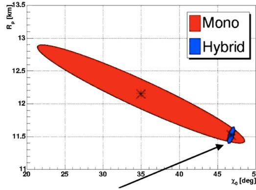
Fig. 31. Error ellipses for geometrical reconstruction of a fluorescence detector.
