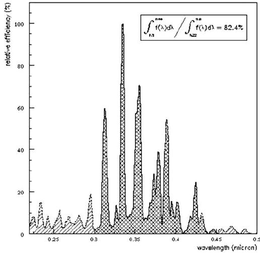
Fig. 20. Fluorescence spectrum in nitrogen measured by Bunner
