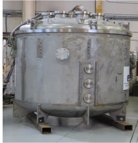
CAPTAIN: “Cryogenic Apparatus for Precision Tests of Argon Interactions with Neutrinos”
