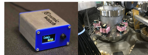
Cosmic watches are used for tagging muons
