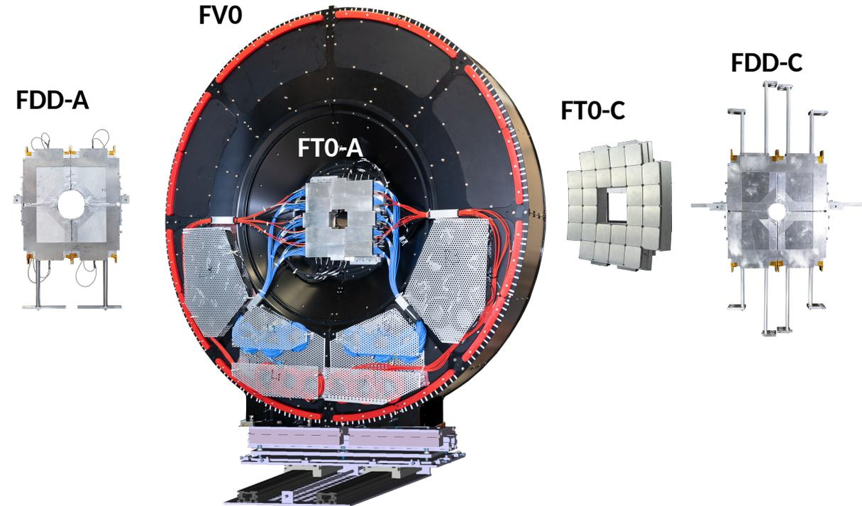
All sub-detectors have a **laser calibration system** and common **Front-End Electronics** and **Detector Control System**.
