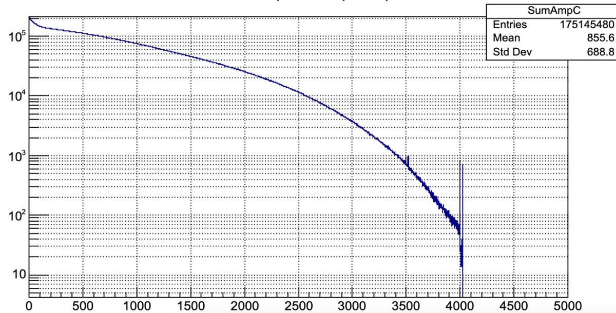
The performance of the side-A and -C shows different amount of charge, i.e., multiplicity. The reason of the high multiplicity in C-Side as well as the saturation has to be understood.
