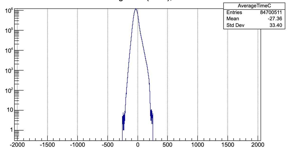
The position of the mean is dependent on the IP position vertex, which can variate on time.
