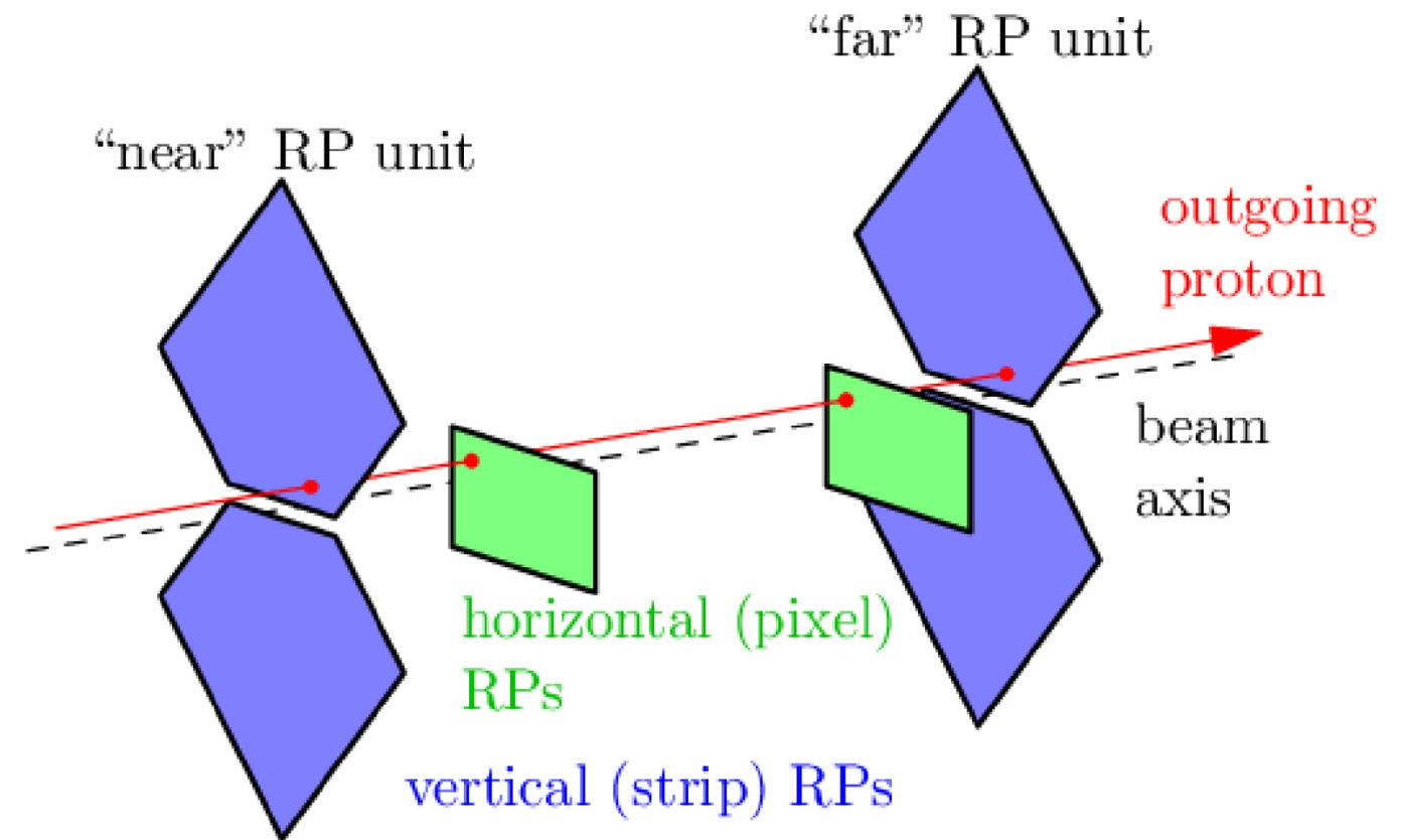
There are six pixel layers in each Pot, each with dimensions of  $100 \times 150 \mu\text{m}^2$ , providing high granularity. The resolution is less than  $30 \mu\text{m}$  and, to optimize both resolution and efficiency, the layers are rotated by approximately  $18^\circ$ .
