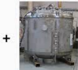
CAPTAIN - "Cryogenic Apparatus for Precision Tests of Argon Interactions with Neutrinos"
