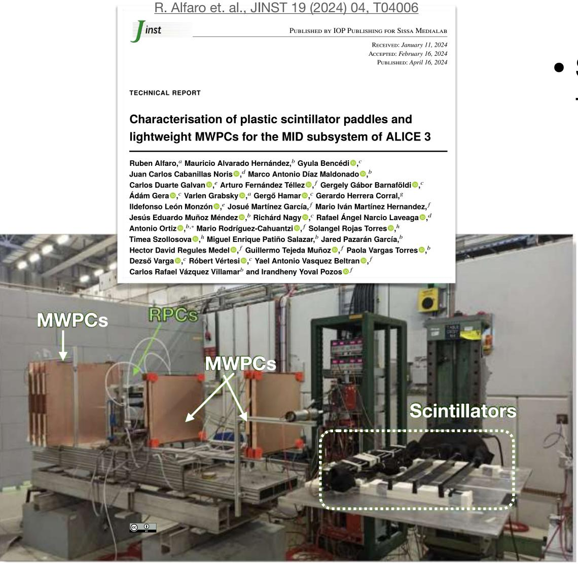
Scintillators and MWPCs prototypes were tested at the CERN T10 test beam facility
