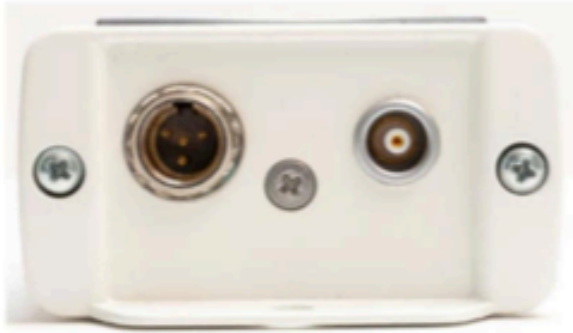
Fig. 5 A7501PB Front panel, LEMO HV and 4-pin Mini XLR connectors for Auger IMON
