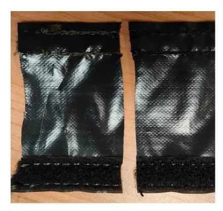
The string is destroyed after an equivalent time of exposure 10.2 months at Malargue with an uncertainty of 20%. This result is well in agreement with the experimental evidence in the field.
