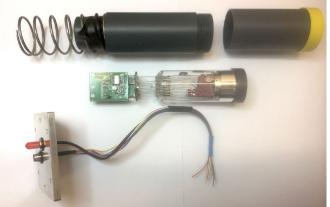
Hamamatsu R9420 eight-stage dynode linear up to 120 mA with modest gain of 5.0X10<sup>5</sup>
