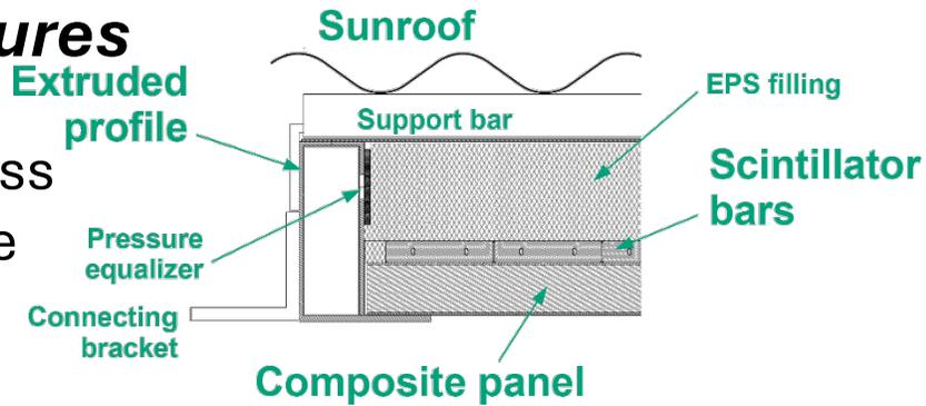
Combination of aluminum bars and composite panel.
