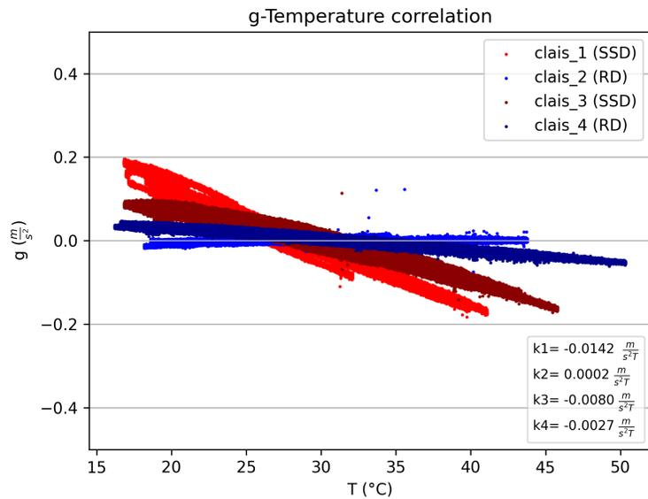
The g modulation can be correlated to thermal winds, even though it differs from sensor to sensor.
