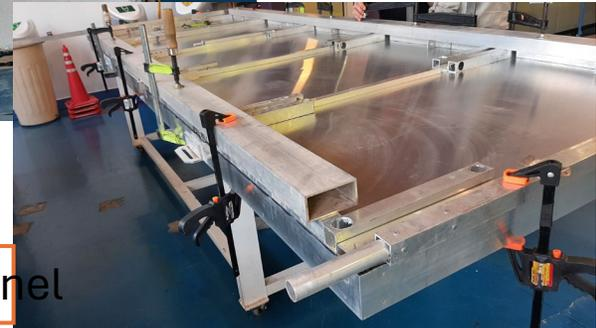
Some difficulties to optimize the curing given the presence of the bars on the upper panel
