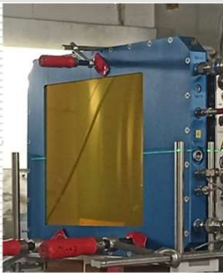
Large area Parallel plate Ionization Chamber
