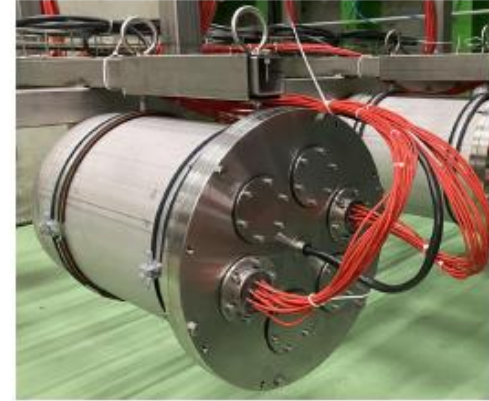
Underwater electronics: Case design and feedthrough
