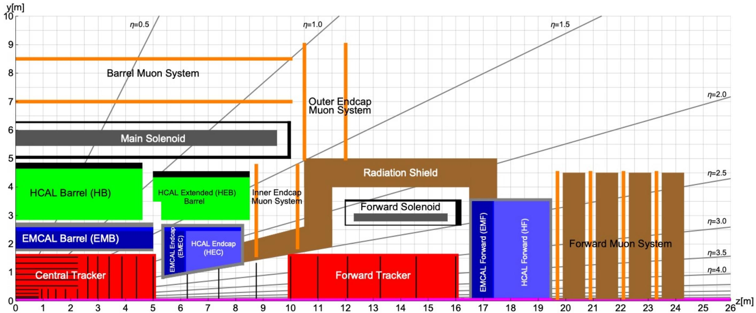
Forward solenoid adds about 1 unit of  $\eta$  with full lever-arm
