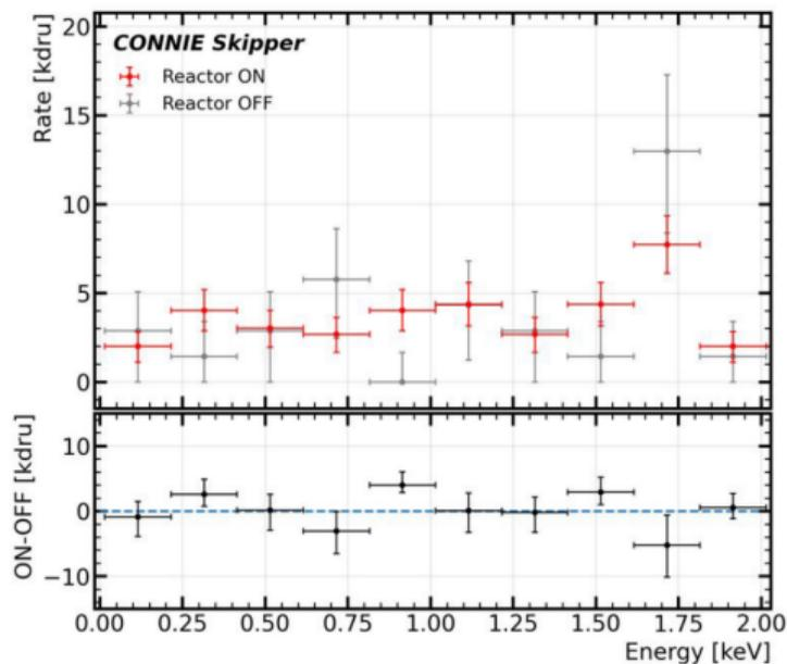
(Top) CONNIE Skipper reactor-on & reactor-off spectra. (bottom) Their difference.
