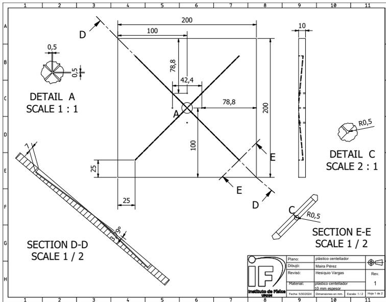
Use wavelength shifter fibers to collect light from a larger surface
