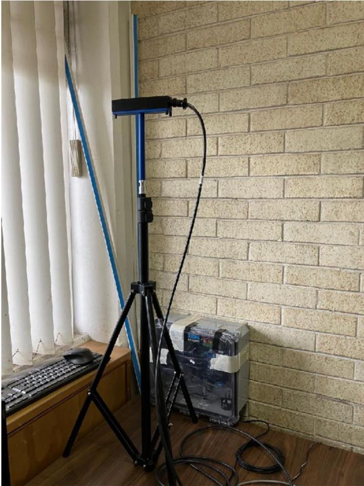
SENSYS FGM3D - magnetometer
