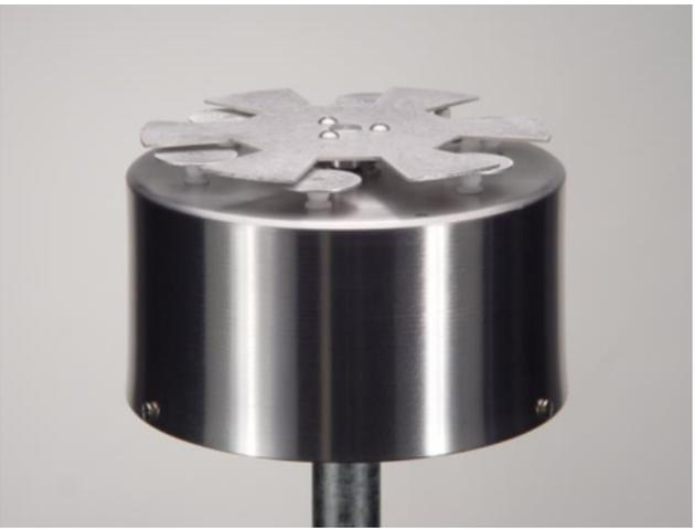
Atmospheric Electric Field Monitor (Field Mill)
