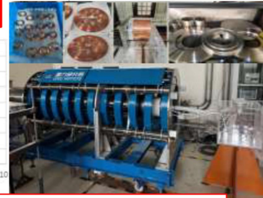
CEPC collider ring 650MHz klystron development in TDR phase
