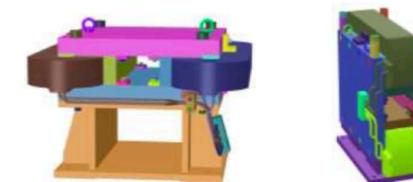
Dual aperture quadrupole: block iron core and new cooling and power line design in EDR
