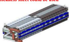
C) Studies on dipole+sextupole combined booster magnet: design and mechanical design completed
