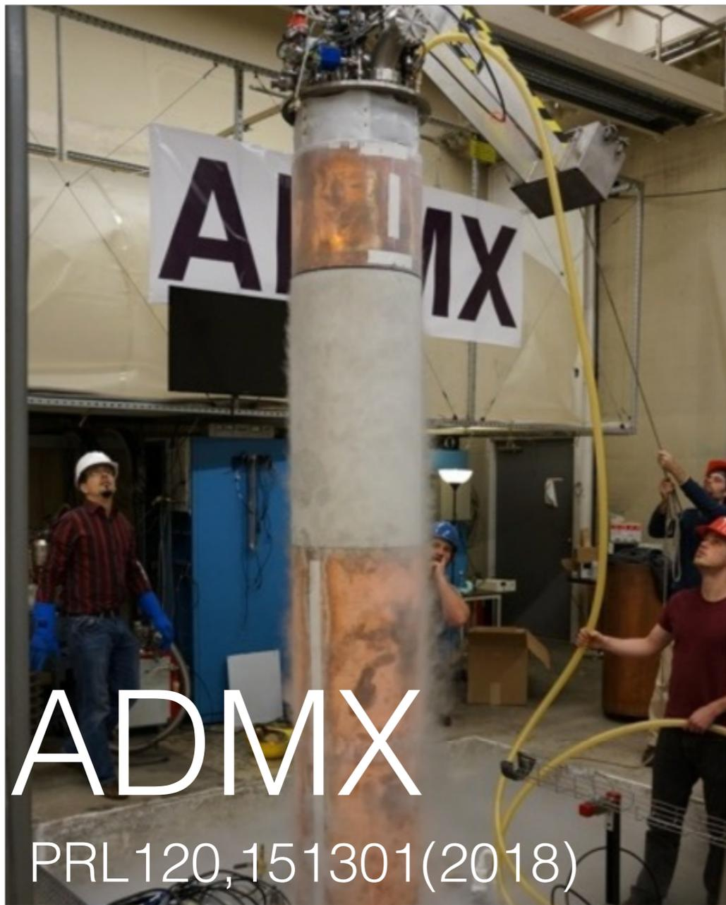
Axion haloscope, uses a strong magnetic field to convert dark matter axions to detectable microwave photons.
