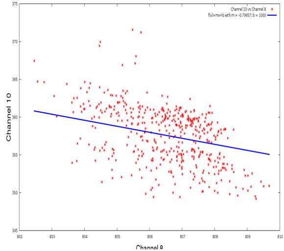
**Figure 6.** Hourly average of the rate (Y axis) and the hourly average of the atmospheric pressure (X axis). The solid line is the least-squares fit with a slope of  $-0.79657$ .
