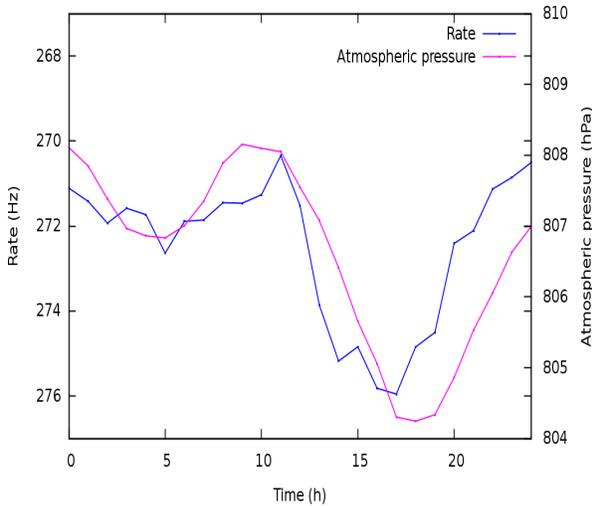
**Figure 5.** Hourly average of the rate of arrival of secondary muons and of atmospheric pressure, showing a clear anti-correlation between them, note that the Y axis on the left side is inverted.
