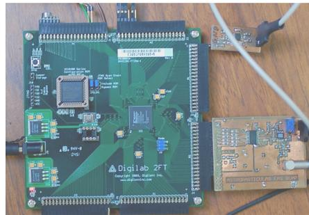
**Figure 2.** FPGA board and the ADC card.
