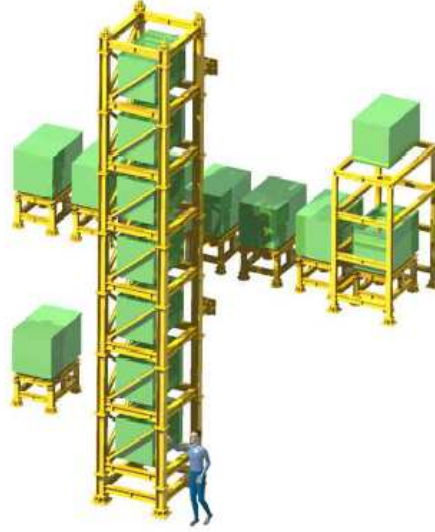
Figure 5. The INGRID detector, consisting of 16 modules.
