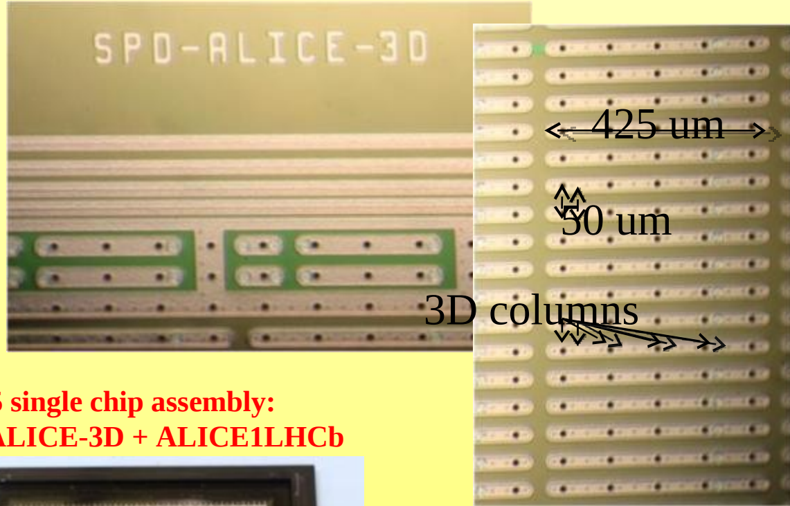
Details of the SPD-ALICE-3D sensor
