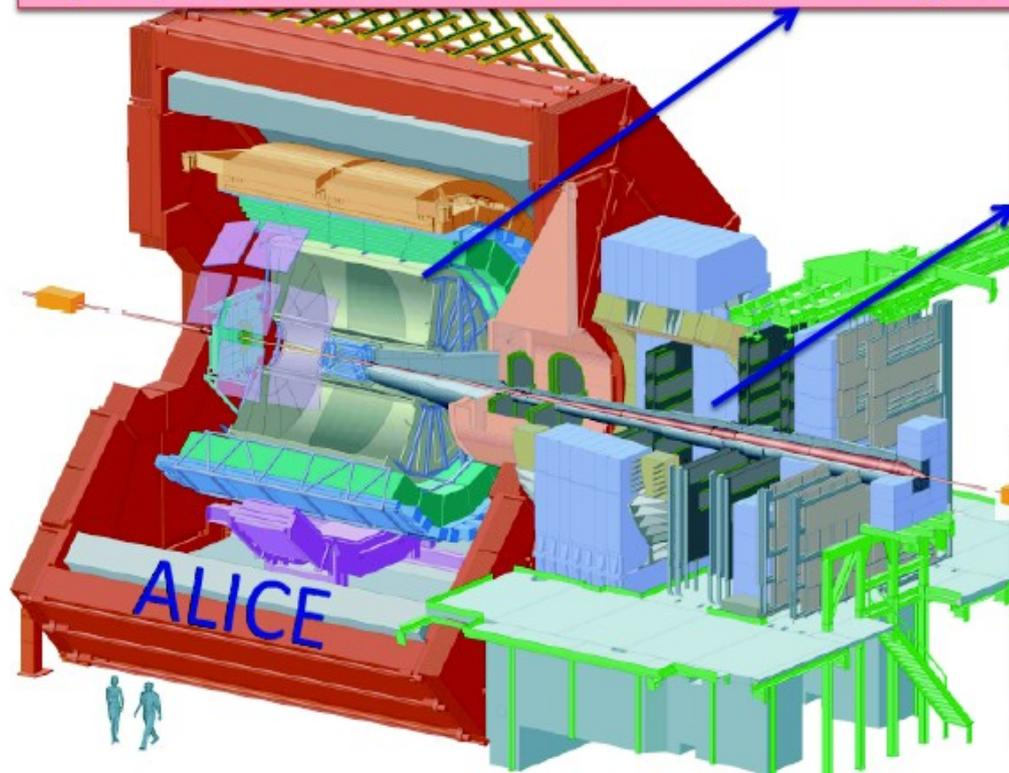
Forward muon spectrometer
