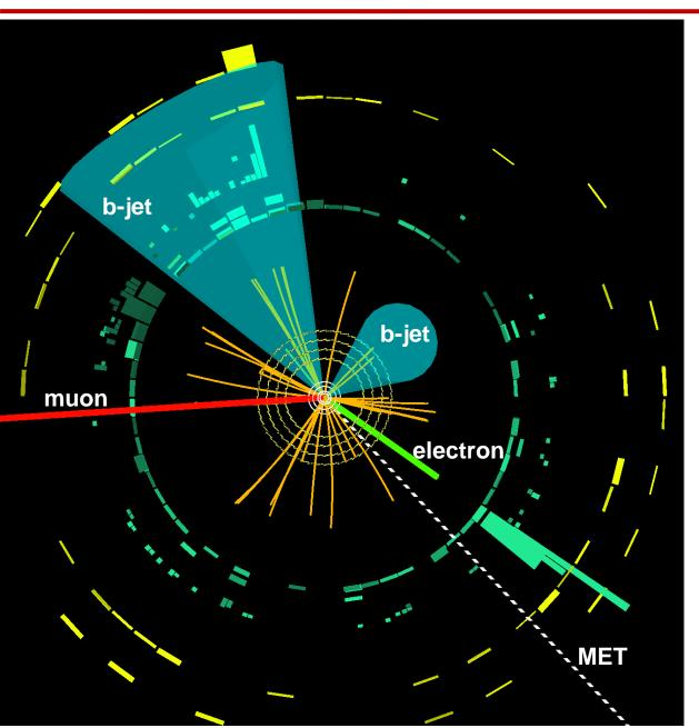
Charged particle tracks reconstructed in the inner detector (orange lines), an electron track (green line), a muon track (red line) as well as the energy deposits in the LAr (green and cyan blocks) and Tile (yellow/orange blocks) calorimeters.
