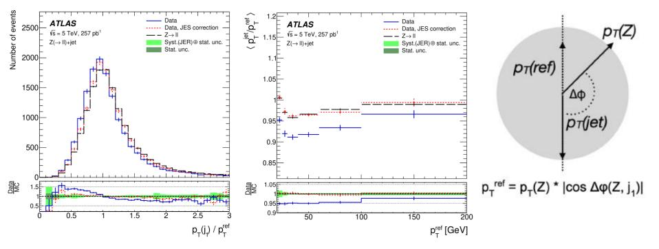
Measure pT(reference) and pT(jet) / pT(reference) in data and in MC simulations: must be balanced in the transverse plane! Then correct the jet energy scale and resolution of data events!
