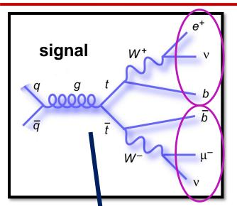
• The dilepton final state arising from ttbar decay is characterised by two charged leptons, two neutrinos and two b-tagged jets
