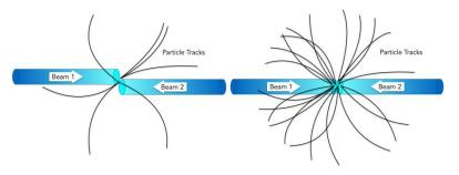
Once a year, LHC proton beams are displaced from their normal position in the horizontal and vertical planes: this method is called a van der Meer (vdM) beam separation scan, allows to map out the beam size and measure ST.
