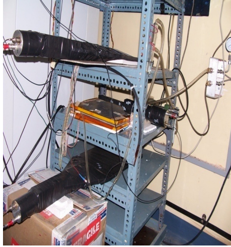
Arrangement of the scintillators and the RPC
