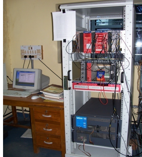
Power supply, front-end electronics and DAQ
