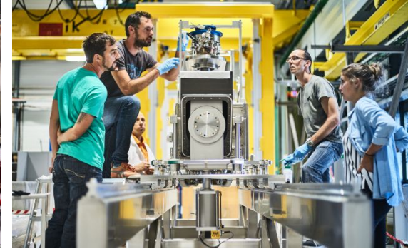
Assembly of the first crab cavity. (Image: Julien Ordan/CERN)
