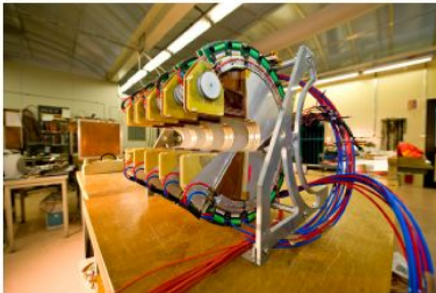
(a) One quarter of the T2 detector on a laboratory table. All five planes are made of a single piece of Gas Electron Multiplier (GEM) detector.
