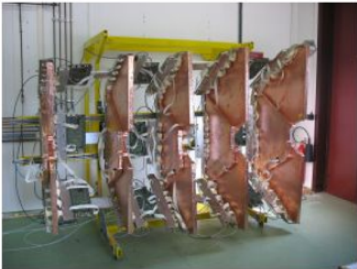
(a) One quarter of the T1 detector stored in the laboratory waiting for its installation. You can see 5 detectors planes surrounded by the read out electronics. All five planes are made of three individual Cathode Strip Chamber (CSC) detectors.
