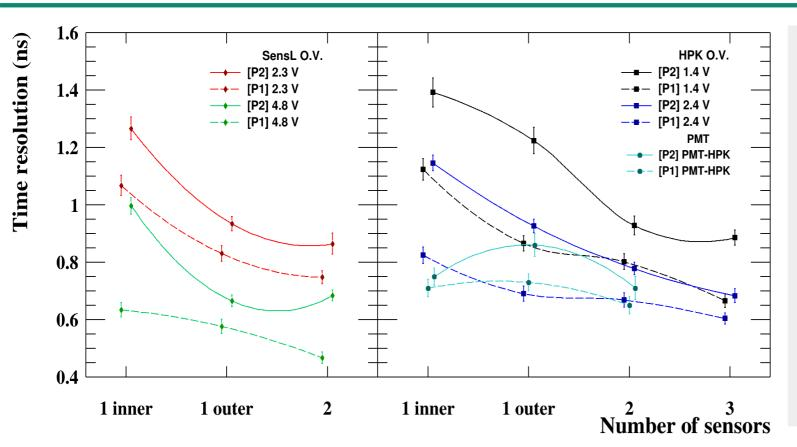
photodetection The efficiency (PDE) of the SiPM increases as a function of the overvoltage. We considered two O.V. values for each SiPM and we observed that by increasing the overvoltage the time resolution reaches lower values.
