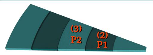
Two prototypes of the were studied using secondary particles of cosmic rays as a radiation source. The time resolution of each prototype depends on the volume (P2 is bigger than P1) due to internal light losses due to multiple reflections and the reduced amount of light arriving in every photodetector.
