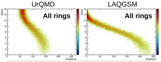
Using the hit multiplicity of all the BeBe detector rings, UrQMD (LAQGSM) predicts a centrality resolution of 45% (34%) for central collision.
