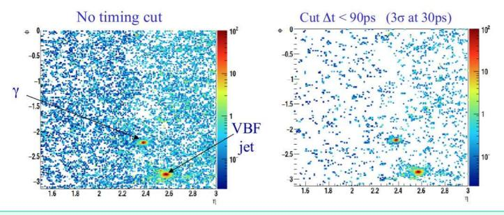
Plots show cells with Q > 12fC (~3.5 MIPs @300mm - threshold for timing measurement) projected to the front face of the endcap calorimeter.
