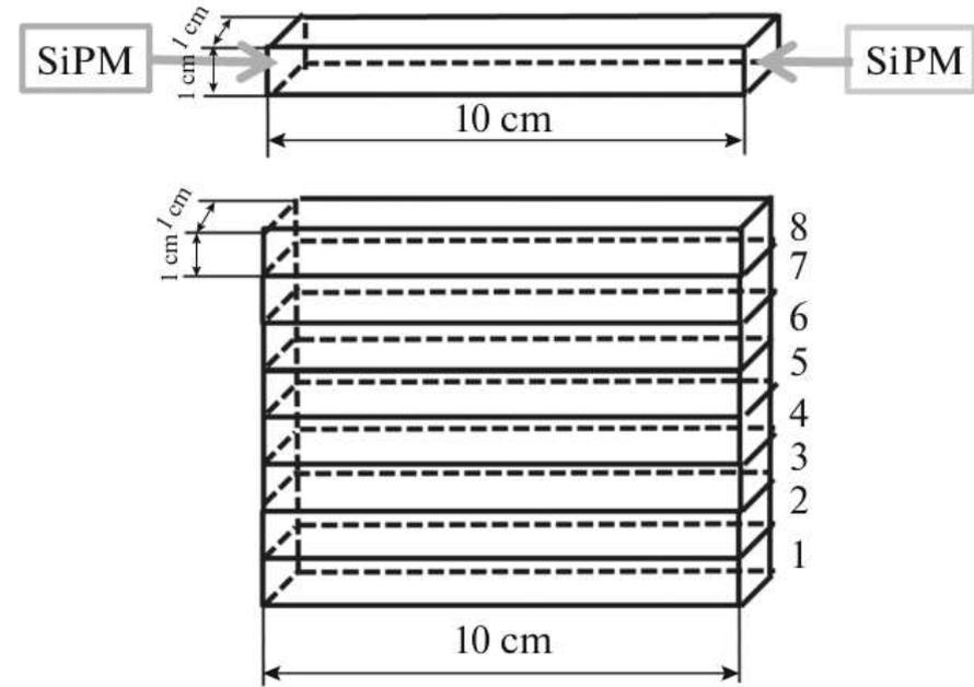
Determining the position of the interaction vertex along the collision axis (Z) in the luminosity detector is calculated from the difference in the time of flight for the left and right halves of the detector. Time resolution around 100ps
