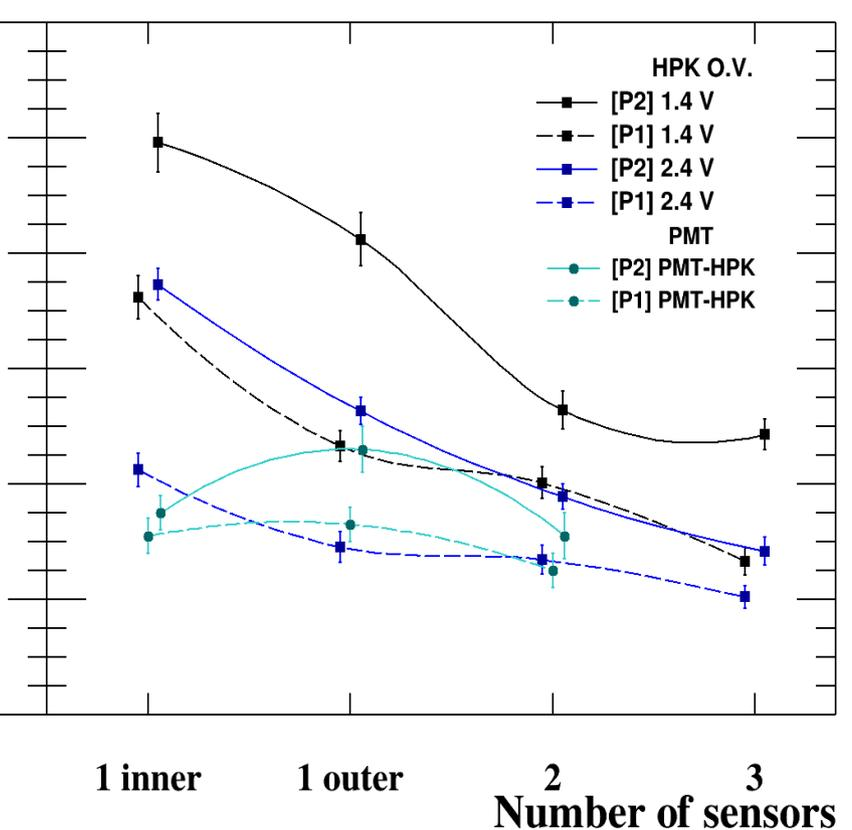
The photodetection efficiency (PDE) of the SiPM increases as a function of the overvoltage. We considered two O.V. values for each SiPM and we observed that by increasing the overvoltage the time resolution reaches lower values.
