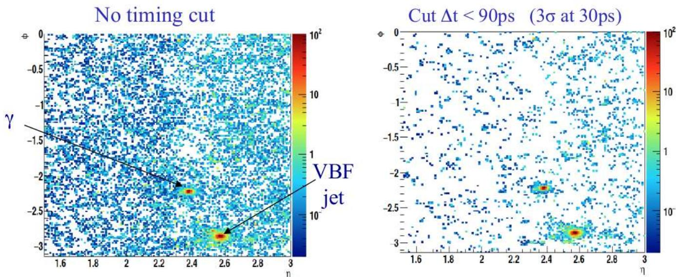
Plots show cells with  $Q > 12\text{fC}$  ( $\sim 3.5$  MIPs @300mm - threshold for timing measurement) projected to the front face of the endcap calorimeter.
