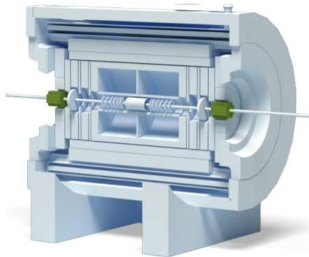
Detector for event centrality and reaction plane measurements with potential for event triggering  $2 < |\eta| < 5$ .
