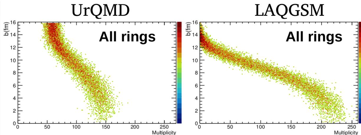
Using the hit multiplicity of **all the BeBe detector rings**, **UrQMD (LAQGSM)** predicts a **centrality resolution of 45% (34%) for central collision.**
