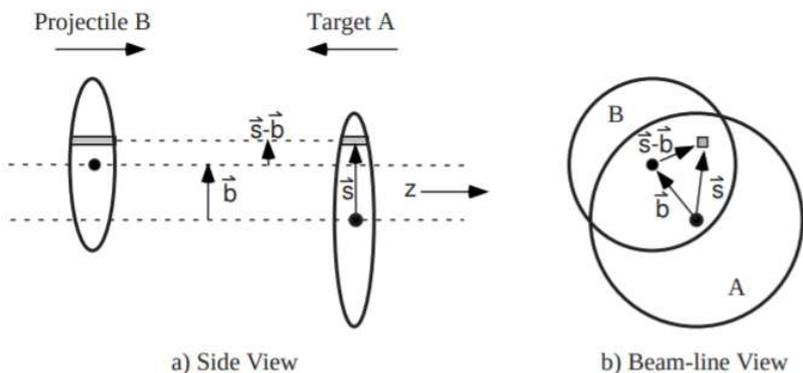
Centrality is a key variable for characterizing the geometric properties of the heavy-ion collisions. We correlated the **impact parameter with the hit multiplicity in BeBe** and looked for the best curve behavior, a linear correlation.
