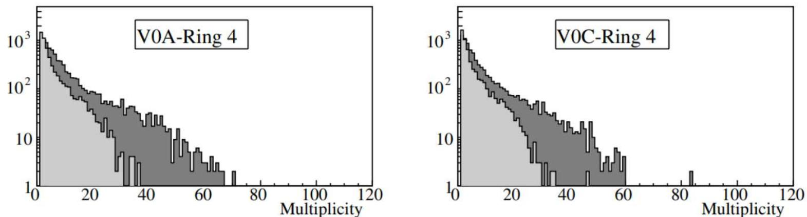
**Figure 3.4:** Charged-particle multiplicity distributions in pp reaction through each ring of the V0A and V0C arrays as given by 7820 PYTHIA inelastic events after transport of particles in vacuum (light grey) and in the ALICE environment (dark grey).
