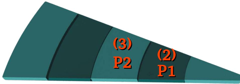
Two prototypes of the were studied using secondary particles of cosmic rays as a radiation source. The time resolution of each prototype depends on the volume (P2 is bigger than P1) due to internal light losses due to multiple reflections and the reduced amount of light arriving in every photodetector.
