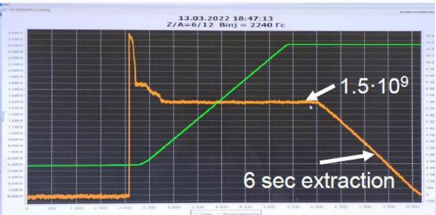
Average efficiency ~ 30%, non-optimum stripping target thickness
