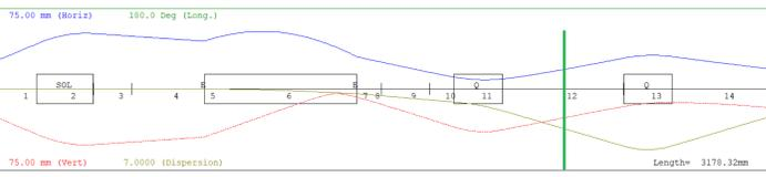
Transverse beam envelopes and dispersion, and the ideal slit position.
