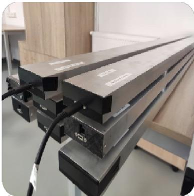
Plastic scintillator in an aluminum housing with an AFE amplification system and a Hamamatsu MPPC photodetector
