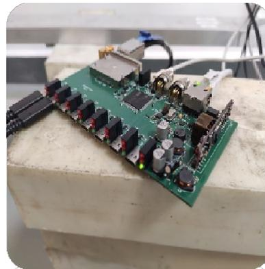
Managed control system for AFE power supplies mounted in boards. Up to 8 boards can be connected once
