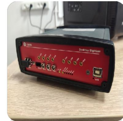
Digital multi-channel amplitude acquirer by CAEN for analysis of received signals
