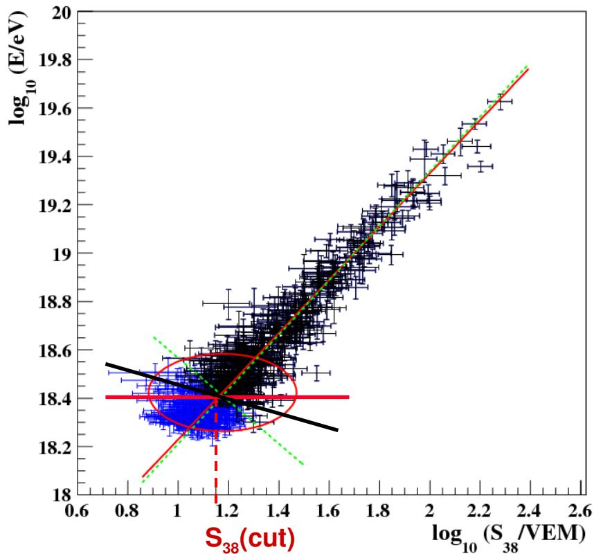
To obtain a surface detector energy calibration curve we need consider the trigger efficiency of the surface detector that is lower than 100% for  $S_{38} \text{ (cut)} \approx 15$  (VEM), and cuts the events below this limit.
