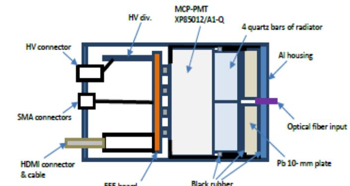
Fig. 4-1. A scheme of the FFD module.
