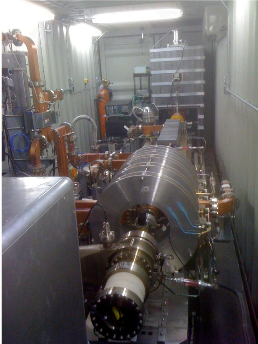
40 MeV electron Linac installed
