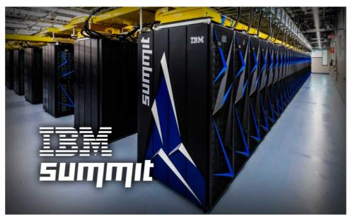
9216 POWER9 22-core CPUs 27.648 Nvidia Tesla Volta GV100 GPUs
