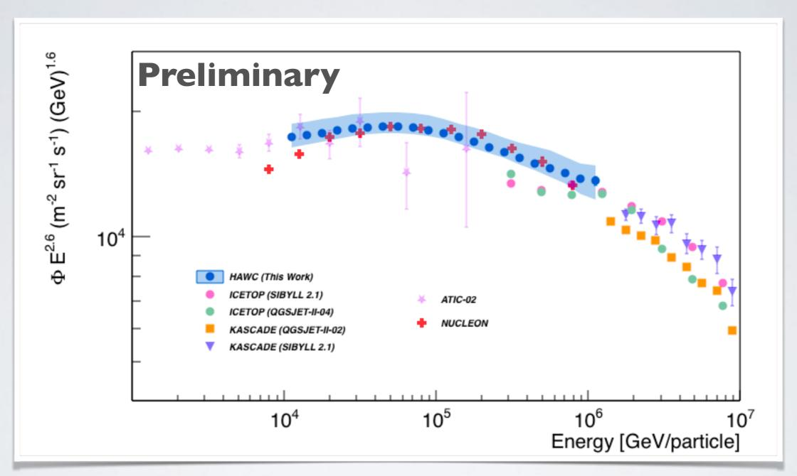
The all-particle cosmic ray energy spectrum obtained in this work compared with the results from ATIC-02 [8], ICETOP [9], KASCADE [10,11] and NUCLEON [12].
