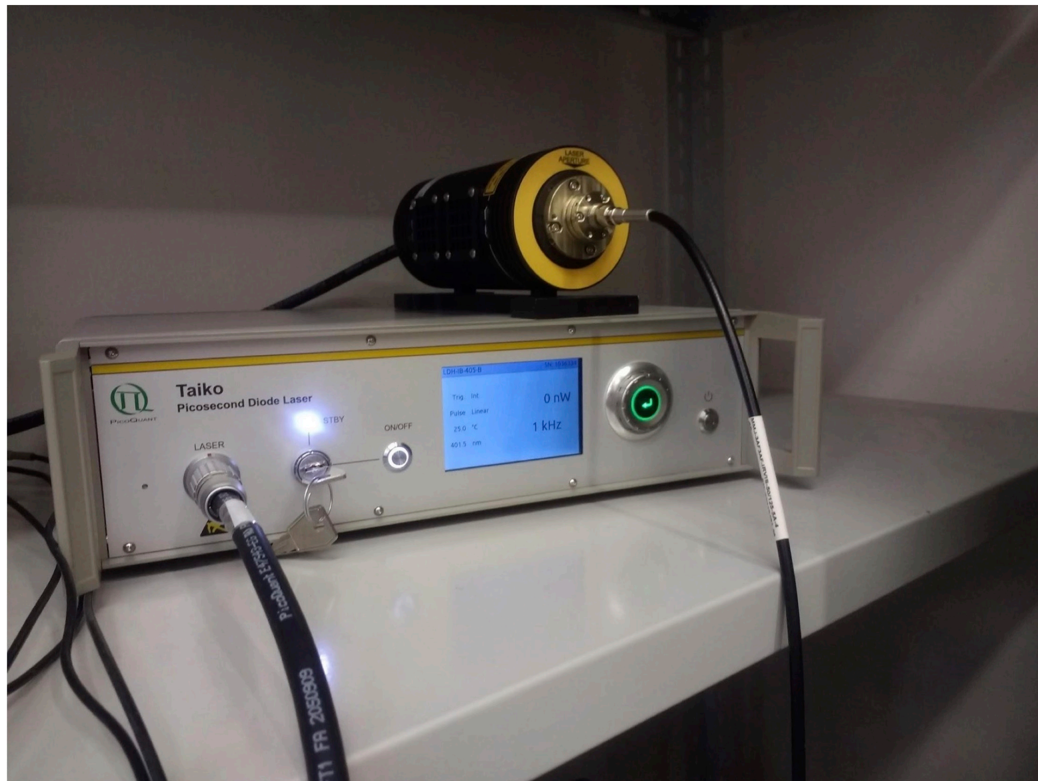
Figure 7. Taiko Laser Driver PDL M1 & Laser Diode Head LDH-IB-405-B
