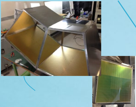
CsI evaporated GEM (inside the gas chamber)
