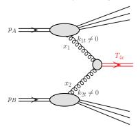
Rysunek: The mechanism of gluon-gluon fusion leading to the production of the  $T_{4c}(6900)$  tetraquark.
