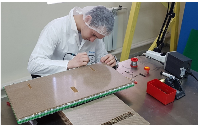
Soldering HV connector and readout pins
