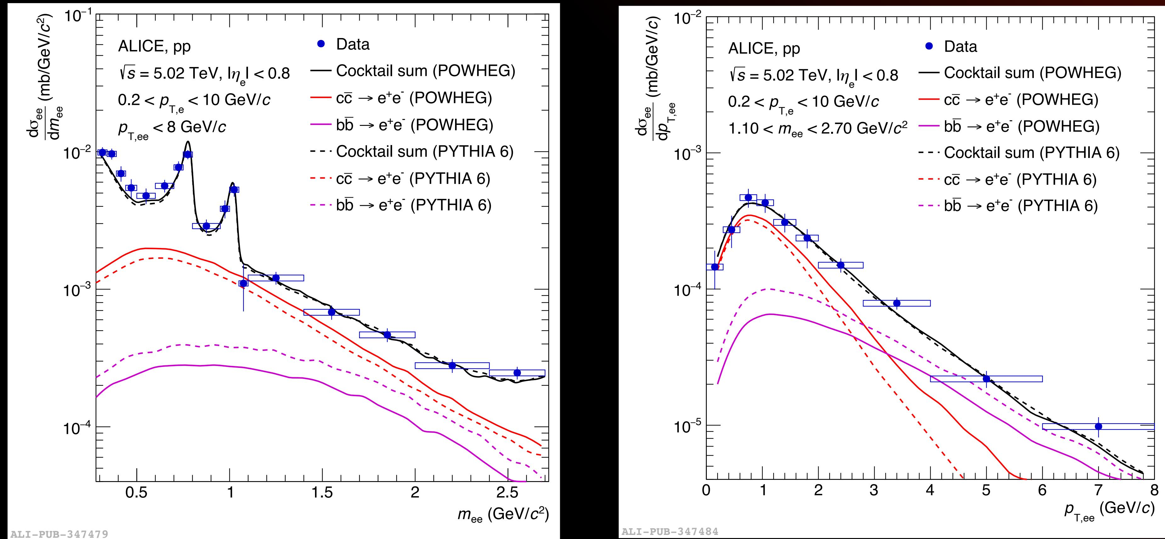
Distinct shape of charm and beauty as a function of  $m_{ee}$  and  $p_{T,ee}$  used to fit data in  $1.1 < m_{ee} < 2.7$  GeV/c $^2$
