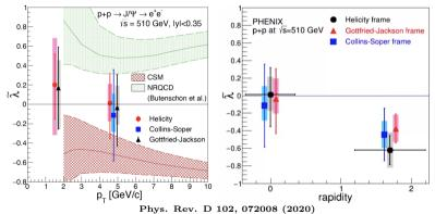
•  $J/\psi$  polarization as a function of  $p_T$  in all three frames is consistent with zero
