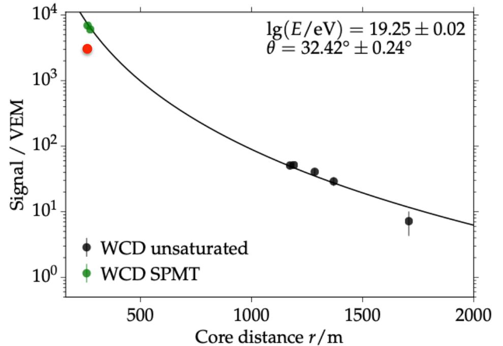
The SPMT allows us to extend the unsaturated measure of the signal very close to the core
