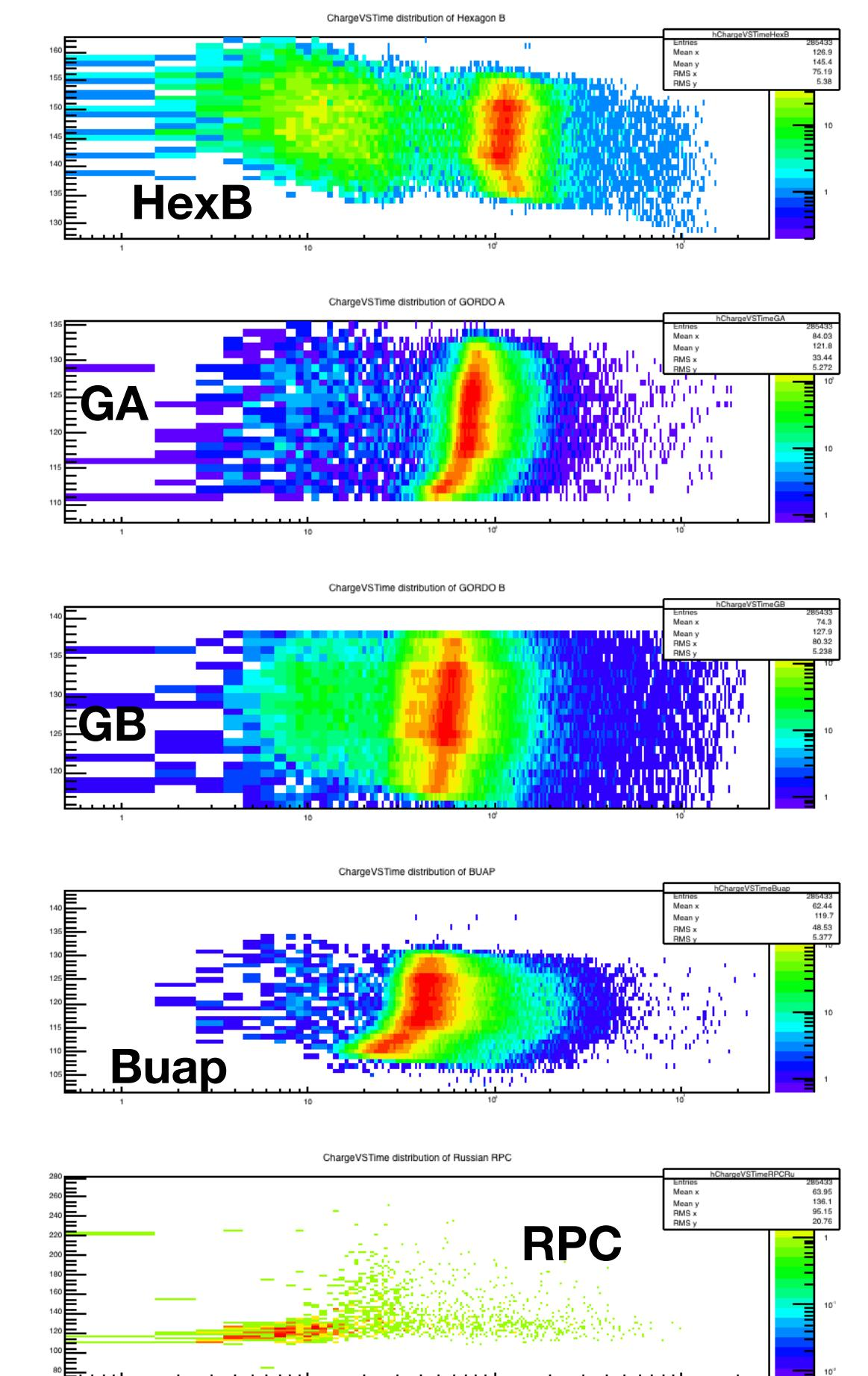
F: RPC voltage 12000 V. First run with RPC in beam test. Possible gas leaking (53% efficiency)
