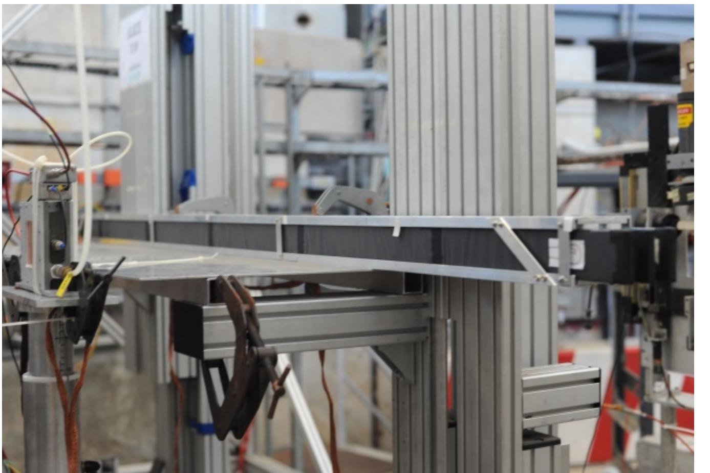
Efficiency measurement along the strips.
